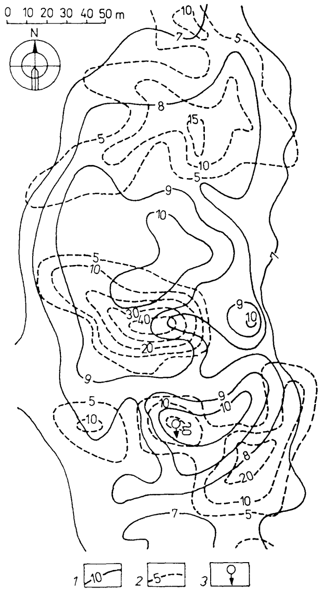
Figure 4.25 Thermometric and gasometric studies of calcium-bicarbonate water near Čačín (according to Husák, in Sborník, 1972). 1 — temperature at a depth of 2 m, 2 — CO 2 content (%) in soil air, 3 — low-temperature spring of calcium bicarbonate water.
